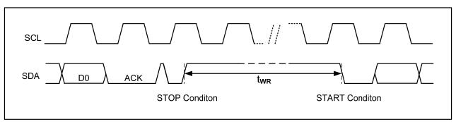
Note: The write cycle time tWR is the time from a valid stop condition of a write sequence to the end of the internal clear/write cycle.
